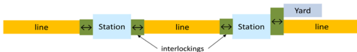
Figure 37. Elements Composing a Railway System Source: SiTI, 2014
